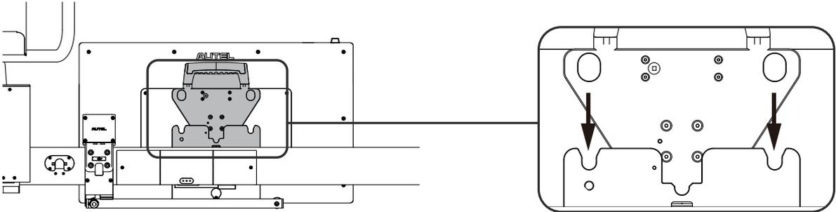
**NOTE:** The two digital target panels can be assembled on either the left or right sliding plate without regard to side.
