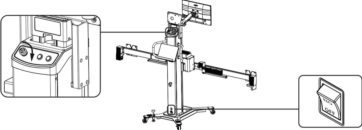
**NOTE:** Check whether the Emergency Stop button is pressed down inadvertently. If so, rotate the button clockwise to release it.
